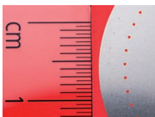
Picture 9: measuring disc with 40µm borehole
