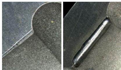
Picture 7: crack in the edge Picture 8: repaired edge before afterwork treatment
